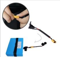
**2<sup>nd</sup> Way**: Connect the charging cable to battery port
