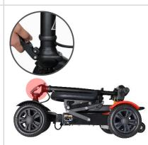
Seat released and could be folded Grip the back of seat and lift upward a little, push Release the handle forward and press downward at the same time.
