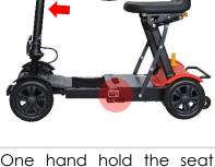
One hand hold the seat, another hand push the steering column forward, then lock both sides handles
