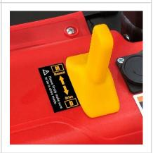
Drive-Manual mode switch (Please switch to Drive mode before driving)
