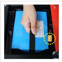
**2<sup>nd</sup> Way**: Pull out the plug and then lift up the battery from box
